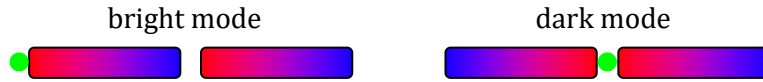
Figure 4.3: Two LSP modes in a nanorod dimer: bright (bonding) and dark (anti-bonding) mode. Position of an electron beam, by which the mode is excited, is marked by the green point. Red color corresponds to a positive charge, blue color to a negative charge.
