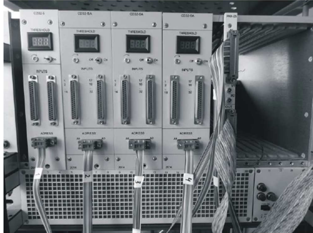
Figure 5. Encoding system “1 from 128” for rear DSSD strips in the individual CAMAC bin
