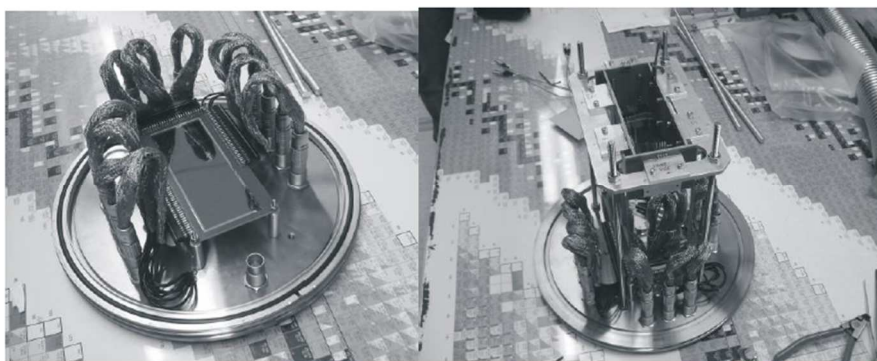
Figure 1. The assemblage of the new DSSD ( 48 \times 128 strips of 1 mm width) with 48 \times 128 \text{ mm}^2 active area in focal plane and of six side SSSD
