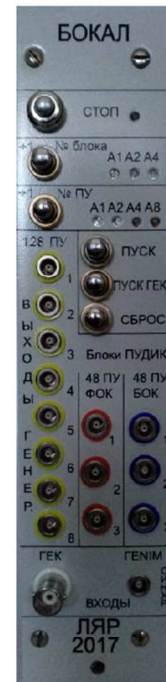
Figure 3. Front view of the module BOKAL (Block for the Organizing of the CALibration)
