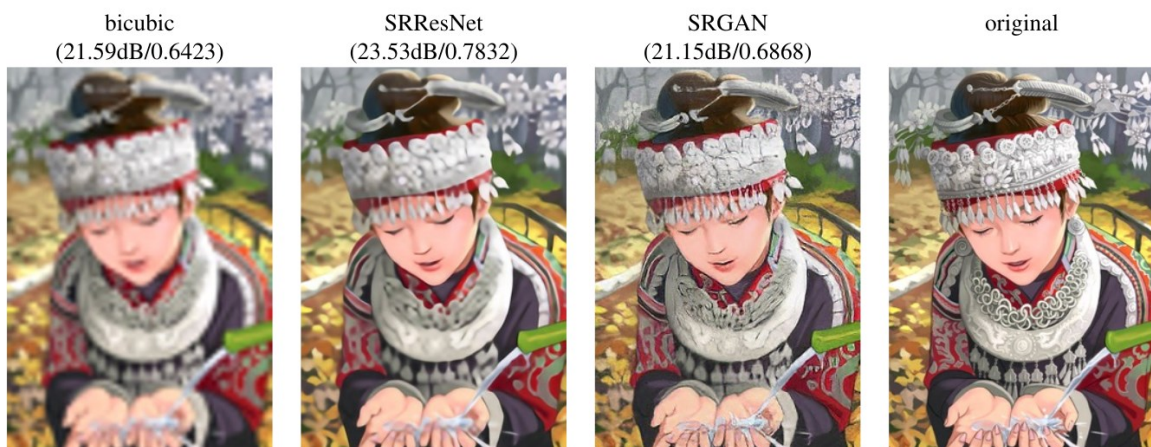
Fig. 2-9 Left to right, Bicubic Interpolation deep residual network, deep residual generative adversarial network, original high-resolution image. Corresponding PSNR and SSIM in brackets (4x upscaling) [6].
