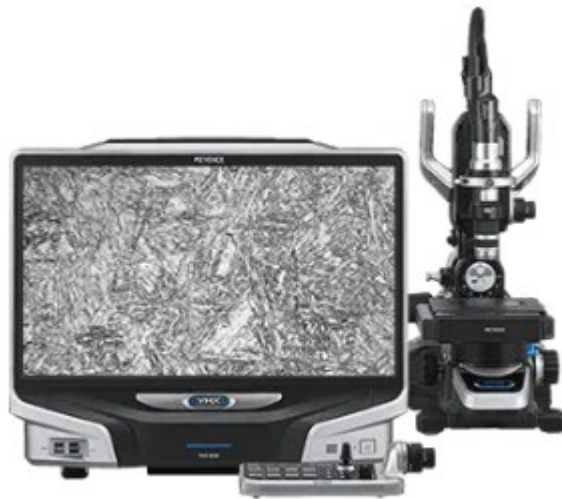
Fig. 4-3 Digital microscope Keyence VHX-6000[27].
