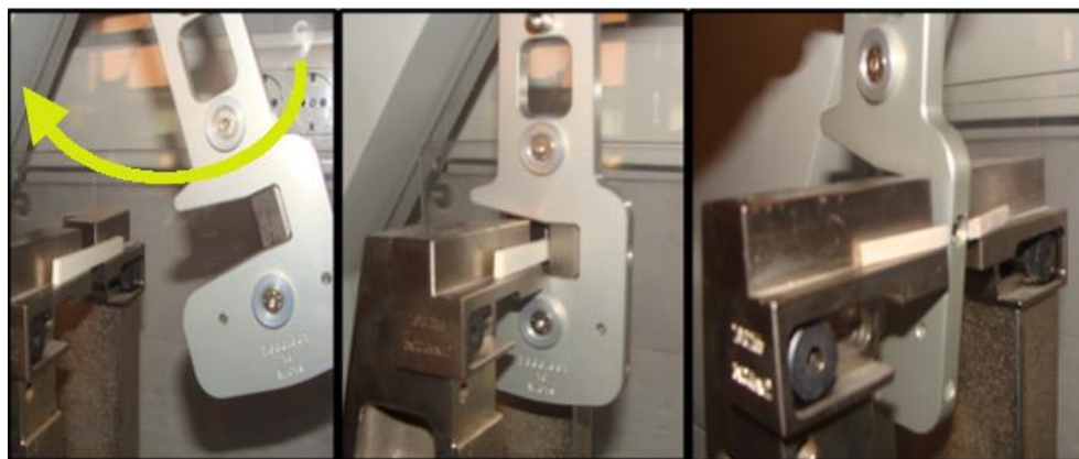
Figure A3. Process of impact test for measuring impact energy absorption to break antler (Photo: Jamil Cappelli).
