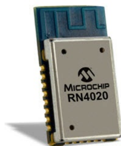
Obr. 9.5: Bluetooth modul Microchip RN4020
