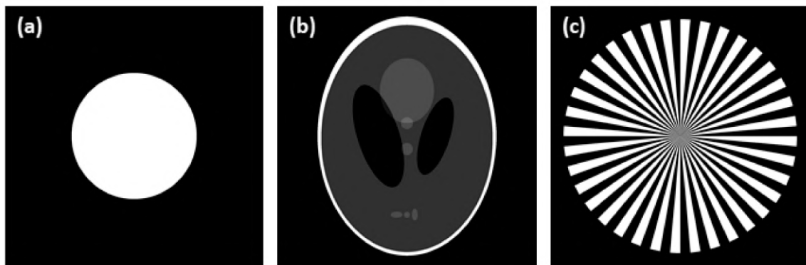
Figure 4. Synthetic data used for testing and validation of all tested methods: (a) ball phantom; (b) Shepp-Logan phantom; (c) Siemens star phantom.
