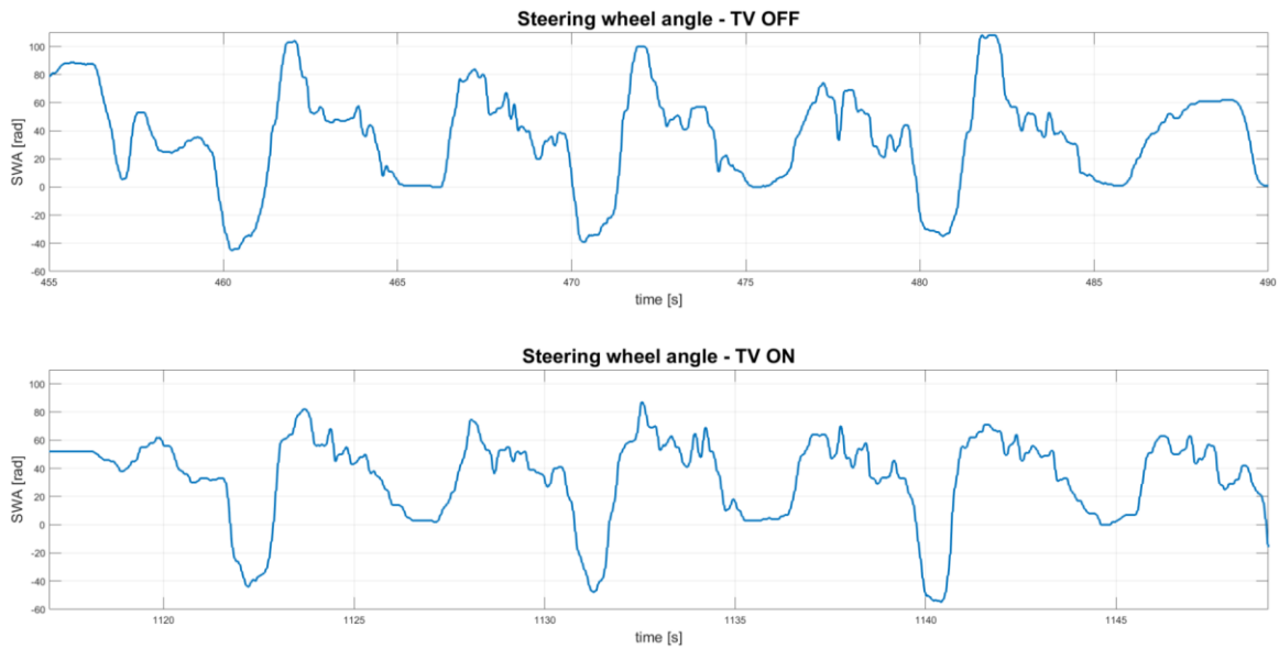
Figure 101 - Steering angle values for a drive without (top) and with (bottom) TV
