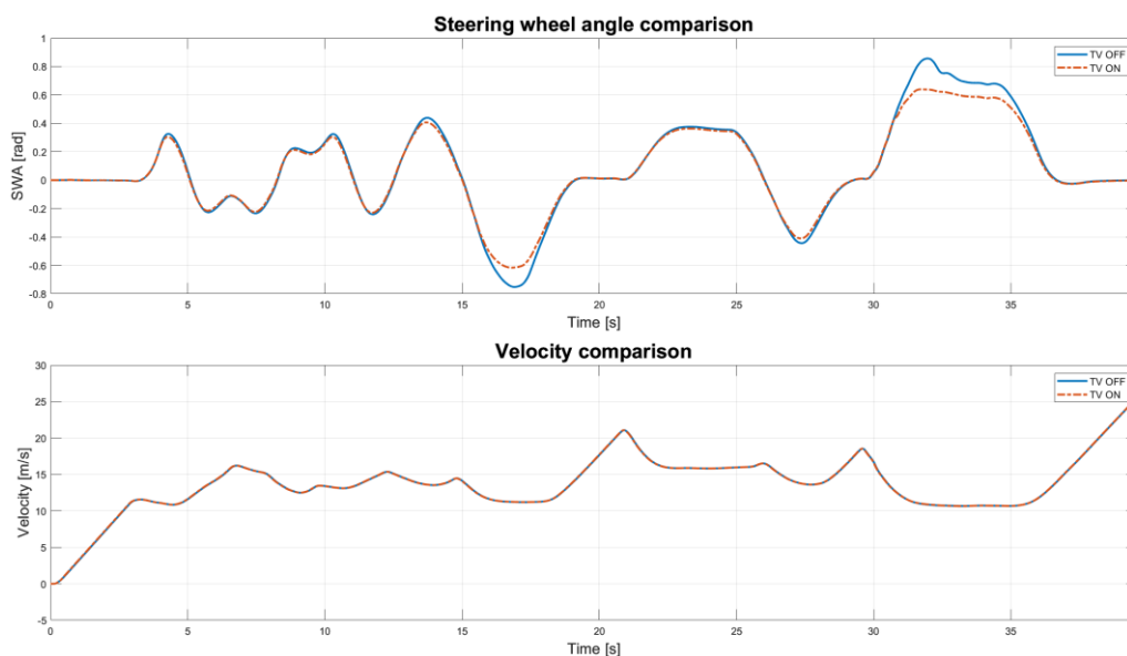
Figure 52 - Steering angle and velocity data from a drive with the custom driver
