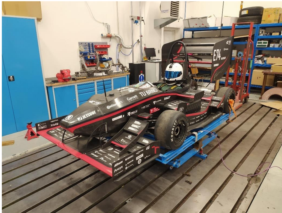
Figure 18 - Vehicle setup for Inertia measurement around Z axis
