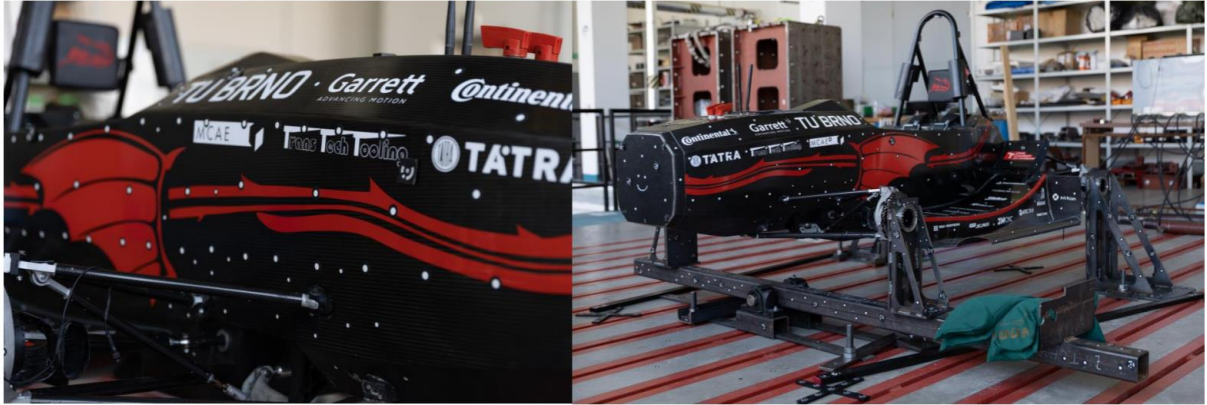
Figure 47 - Validation of the chassis torsional stiffness via a photogrammetry method [21]
