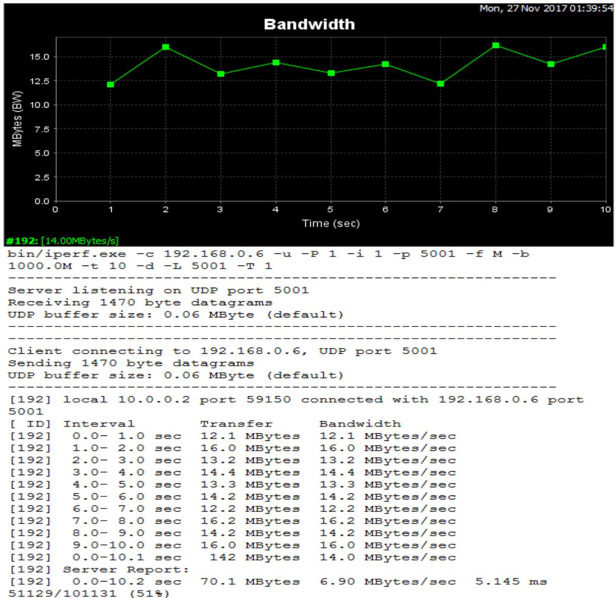
Figure 13 - UDP Mixed Packet Sizes(SRX)
