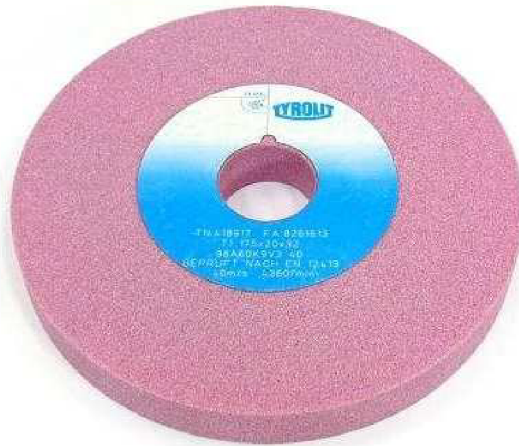
Obr. 2.1 – Kotouč Tyrolit T1 175x6x20 – A98 A60 K9 V [37]
