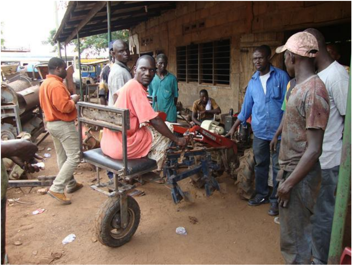
PICTURE 2: Traditional way of modifying power tiller in Ghana
