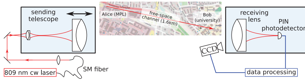
Fig. 1. A schematic view of the experimental set-up. At the sender Alice we use a telescope to expand the beam and adjust its beam width. Subsequently the beam is sent through our 1.6 km free-space link to the receiver Bob. There we use an achromatic lens with a diameter of a = 150 mm and measure the fluctuating transmission using a PIN photodiode detector and an analogue-to-digital converter. To estimate the aperture-to-beam size ratio we use a CCD camera and a screen.
