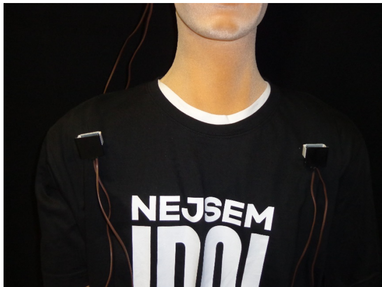
Figure 58. The plate sensor placed on thermal mannequin
