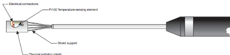
**Figure 65.** The Air Temperature Sensor – INNOVA MM0034
