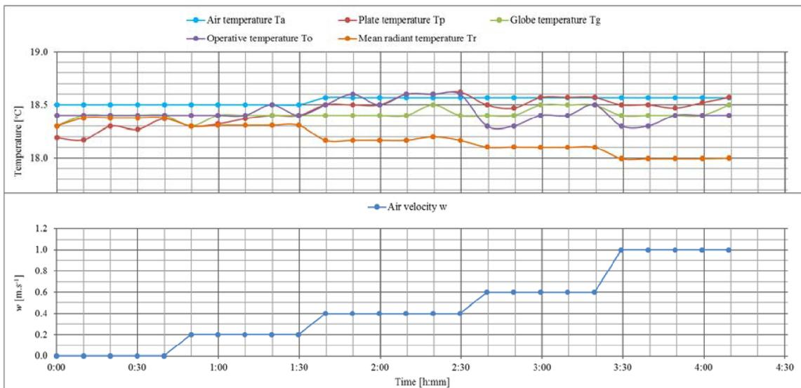
**Figure 73.** Testing the New Plate Sensor (first period)
