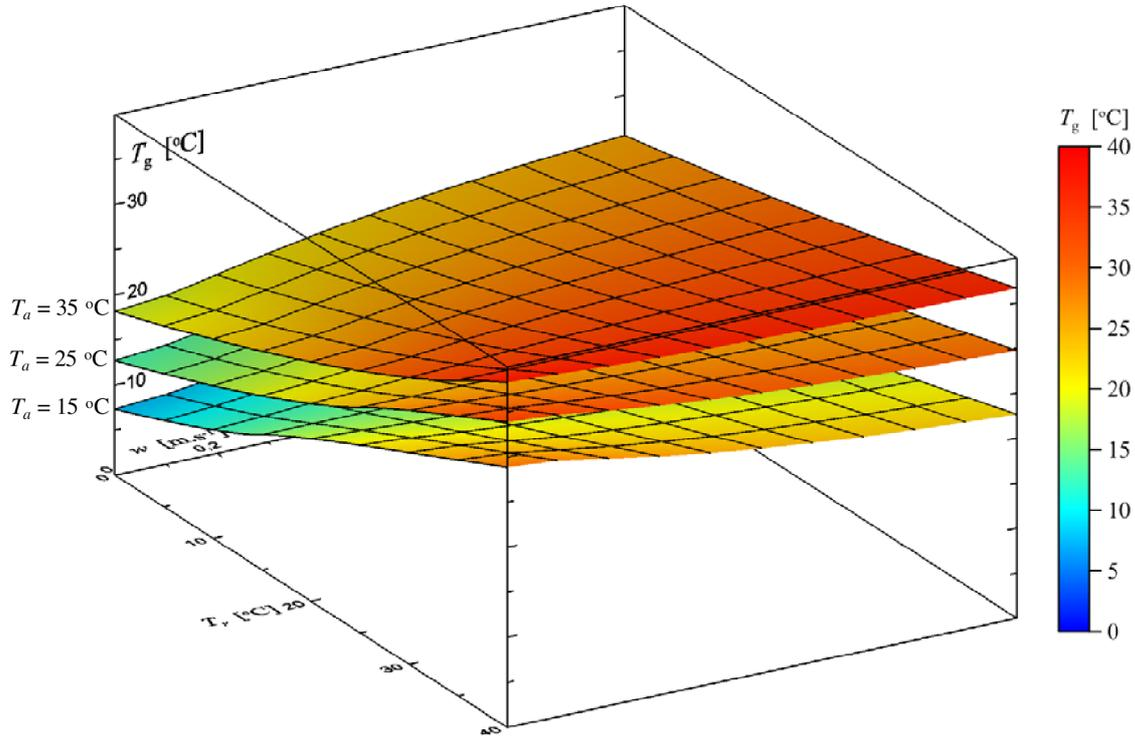
**Figure 16.** The globe temperature function for constant air temperature – Side view
