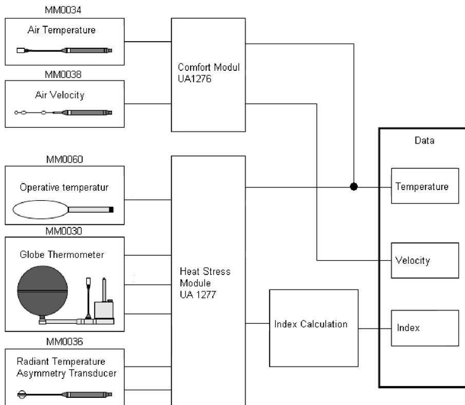
Figure 69. Overview of sensors types used in experiment
