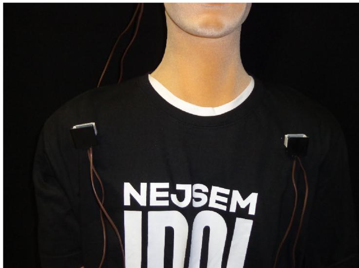
**Figure 58.** The plate sensor placed on thermal mannequin
