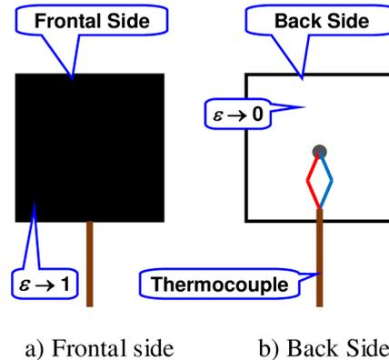
**Figure 29.** The compact plate sensor
