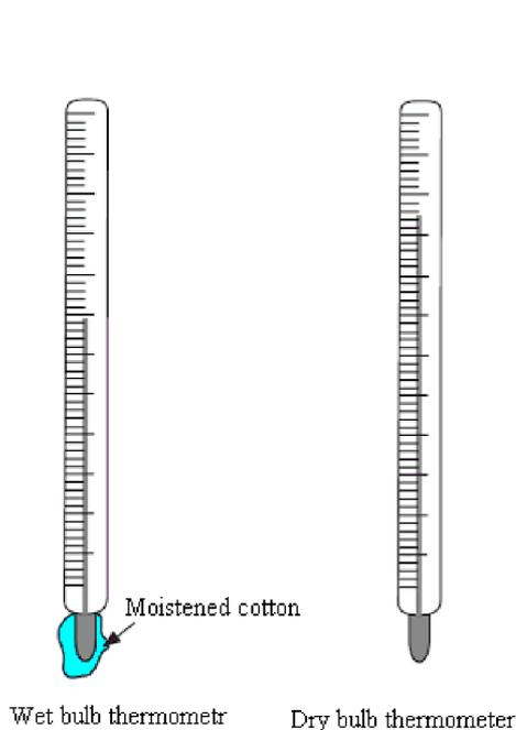
Figure 6. The wet and dry bulb thermometers
