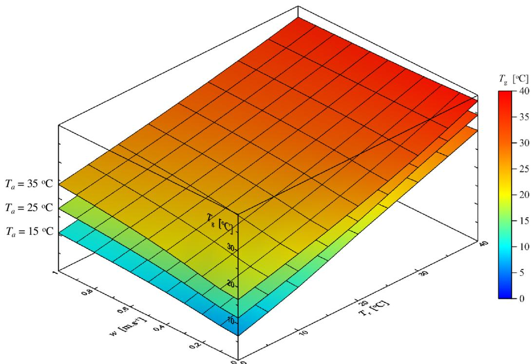
**Figure 17.** The globe temperature function for constant air temperature – Front view
