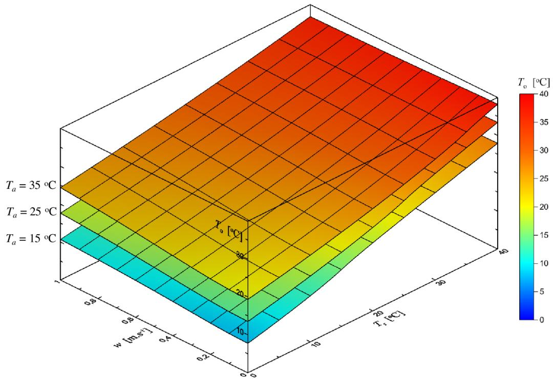
Figure 19. The operative temperature function for constant air temperature – front view
