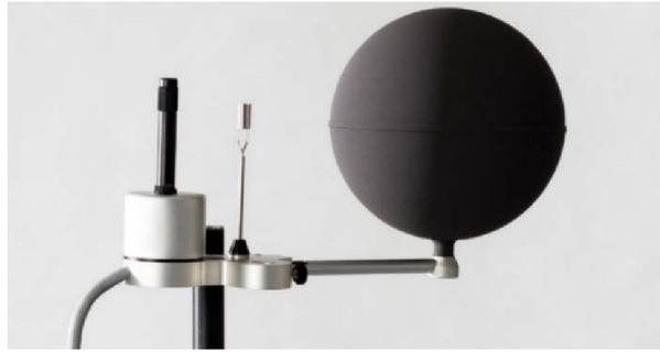
**Figure 64.** The Wet Bulb Globe Temperature (WBGT) Sensor
