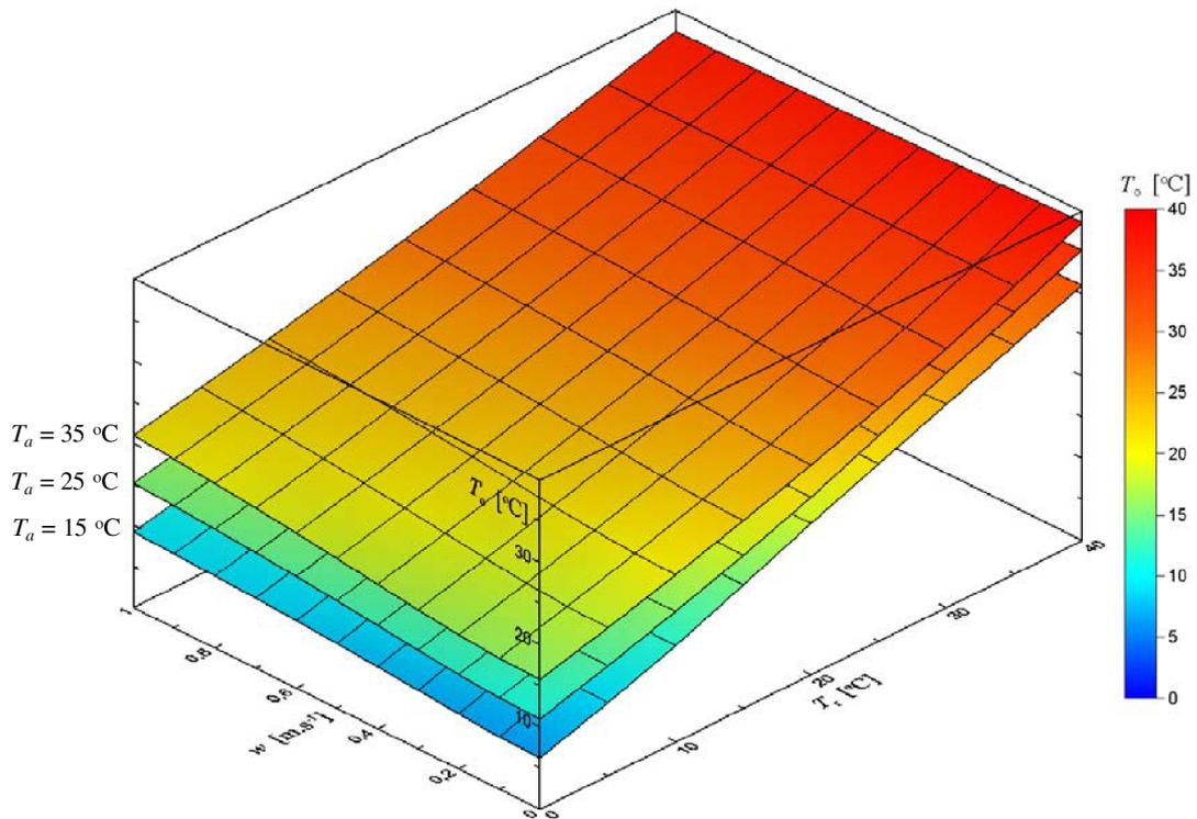
Figure 21. The operative temperature function for constant air temperature – front view
