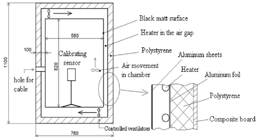
**Figure 61.** Scheme of calibration chamber (Janečka et al. 2011)
