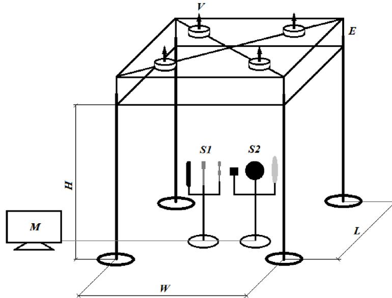
**Figure 60.** Scheme of test chamber: S1 – Set of sensors to measuring humidity, velocity, and temperature of the air; S2 – Set of thermal comfort sensors; V – ventilators with adjustable flow; M – monitor; Chamber Dimensions (W - width, L - length, H- High)
