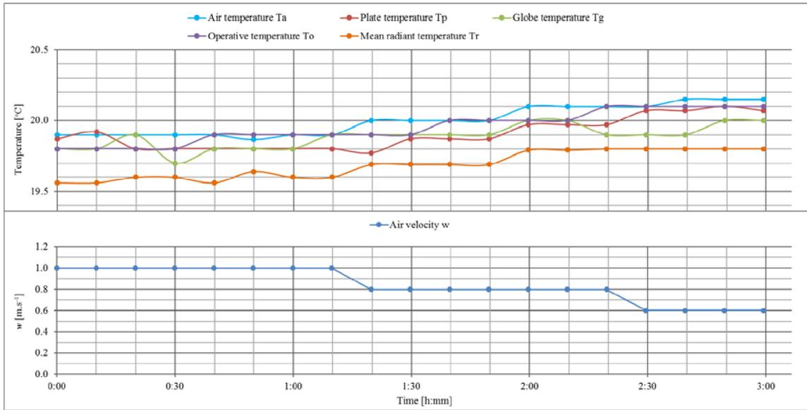
Figure 74. Testing the New Plate Sensor (second period)
