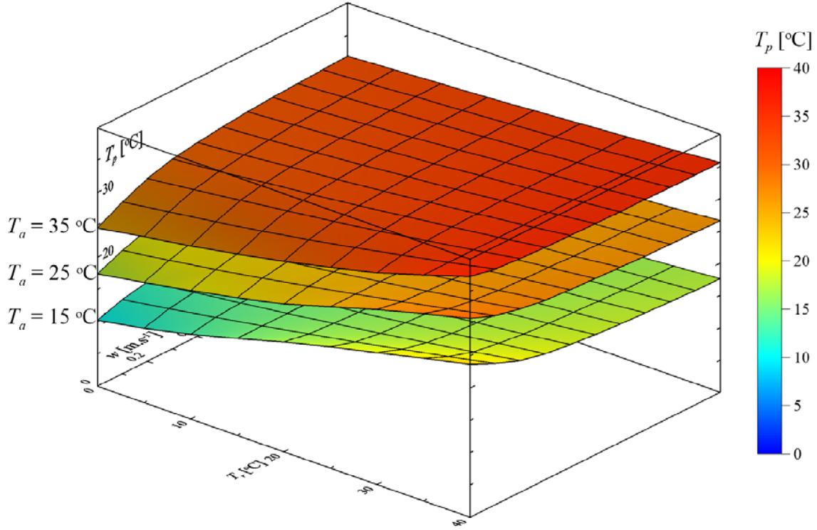
**Figure 31.** The plate temperature function for constant air temperature – side view
