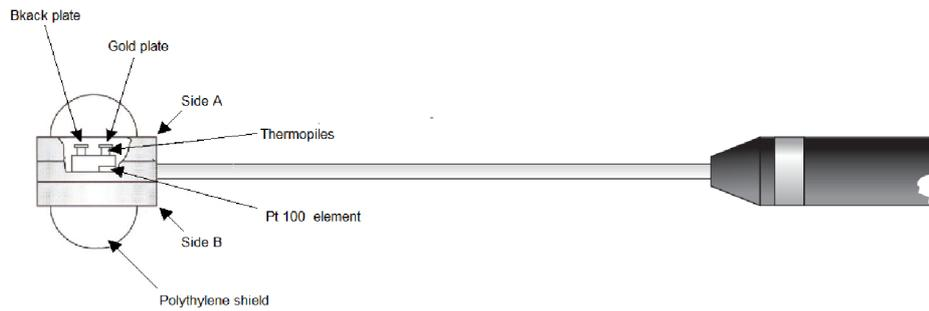
**Figure 66.** The Radiant Temperature Asymmetry Sensor – INNOVA MM0036
