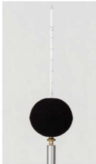
*Figure 11.* The globe thermometer
