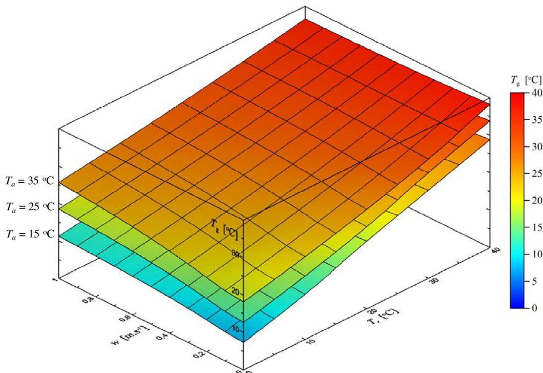
**Figure 15.** The globe temperature function for constant air temperature – Front view
