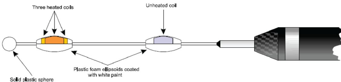
**Figure 67.** Air Velocity Sensor – INNOVA MM0038
