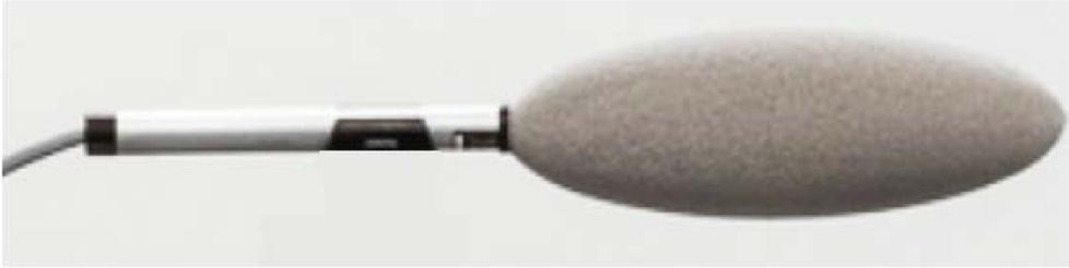
*Figure 68.* The Operative Temperature Sensor – INNOVA MM0060
