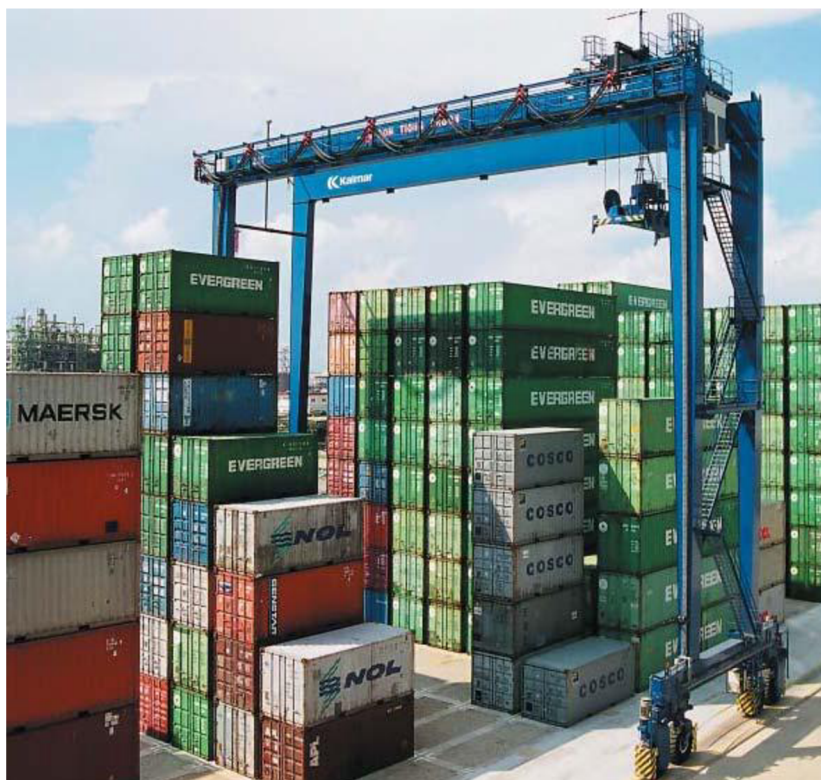
Obr. 27 RTG jeřáb firmy Kalmar [6]
