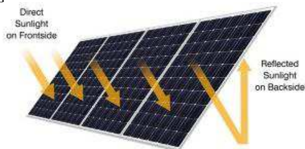
Figure 3-7 Bifacial solar panel [12]
