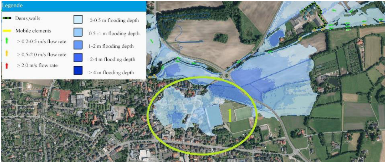
Figure 28. The flood hazard map for the study area with HQ100, where 1, the area of the planned constructions (ELWAS Karte, 2016).
