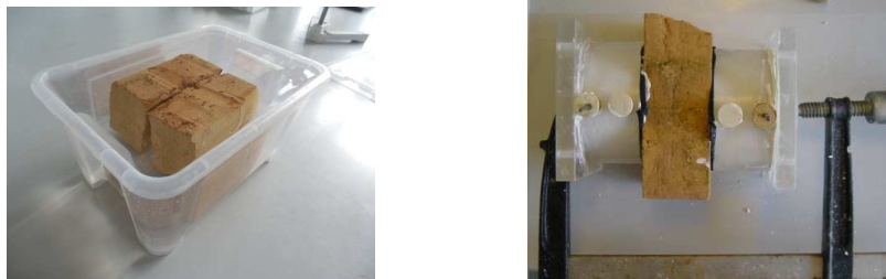
Fig. 6 The used yellow brick contaminated with NaCl solution (left) and the used closed laboratory setup (right). The wrapping is not shown. [14]
