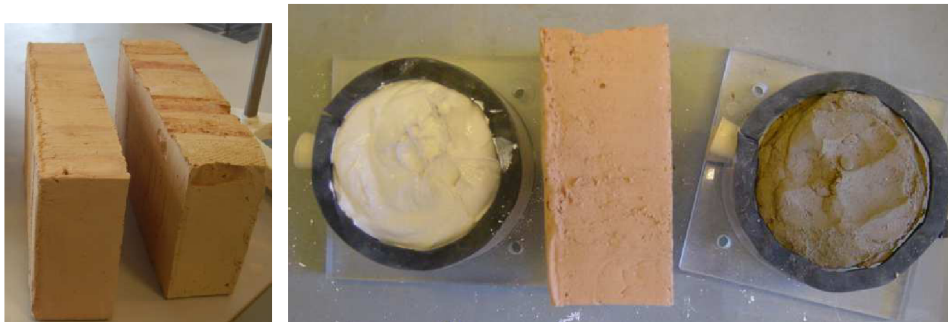
Fig. 3 The used yellow bricks, the clay poultices – the mixture (white), the brick clay (brown); [10]
