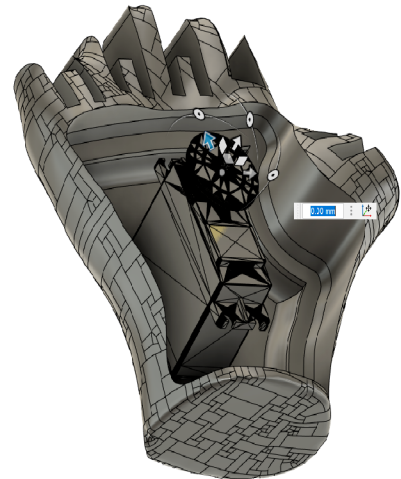
Figure 3.48: Fitting servo model into palm area side view
