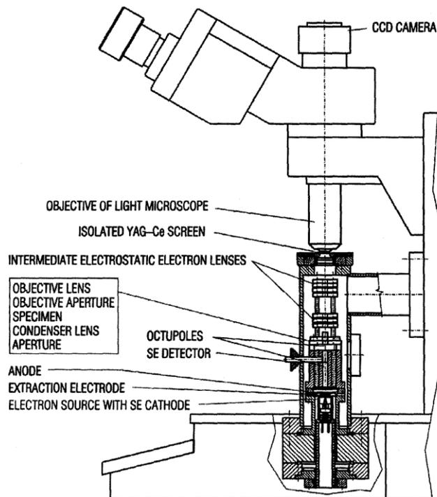
**Fig.2: The scheme of LVEM5 design. In the bottom part of the own electron microscope is placed an electron gun and , the middle part consist of an optical microscope with magnification of 400 times and finally on the very top a slow scan CCD camera detect the formed image.**
