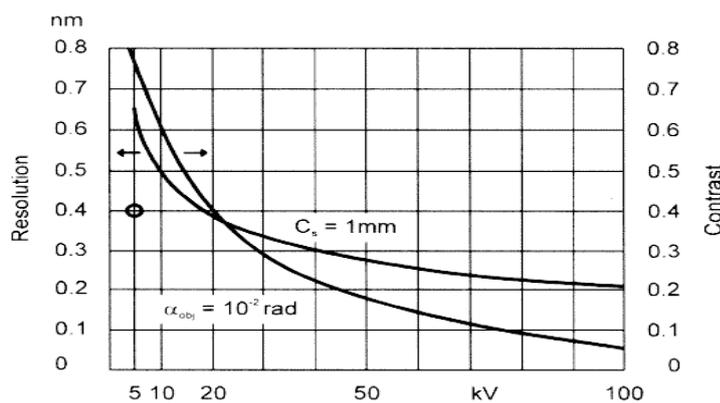
Fig.1: Dependence of resolution and contrast on the accelerating voltage in the transmission electron microscopy. The dependence of contrast holds for a carbon foil 20nm thick. (Delong at al. 2000)
