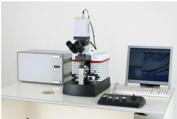
**Fig.3: The LVEM5 multifunctional electron microscope can be placed on a working desktop with no special space requirements.**
