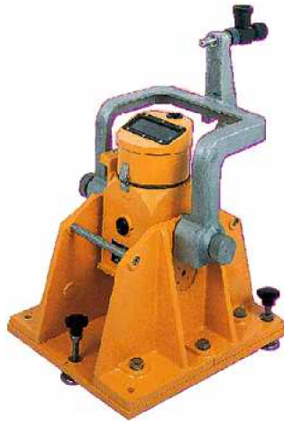
Obr. 6.3 Sky-screen hradlo High Pressure Instrumentation (viz. [8])
