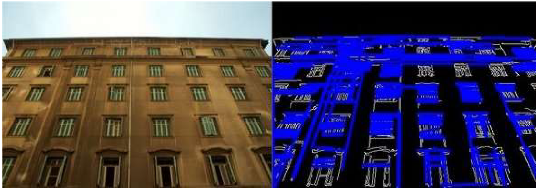
Obr. 15: Randomizovaná Houghova transformace v OpenCV [17]
