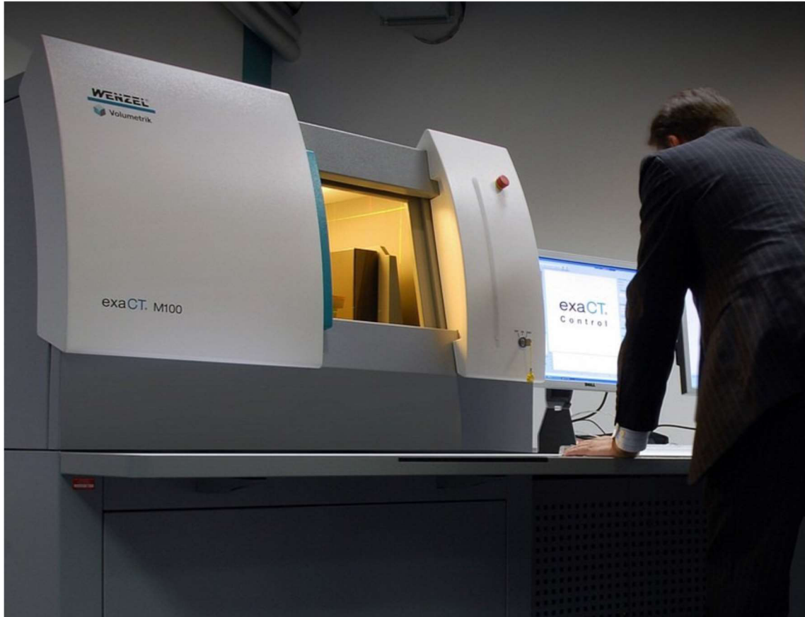
Obr. 7: CT skener Wenzel ExaCT M100 [3]
