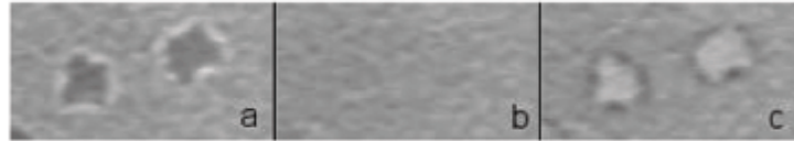
Figure 6. a) positive defocusing, b) in focus (object invisible,) c) negative defocusing
