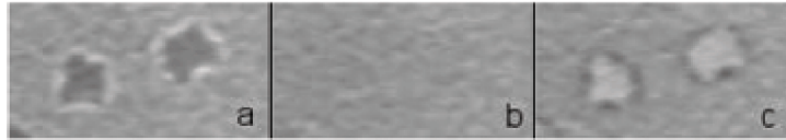
Figure 6. a) positive defocusing, b) in focus (object invisible,) c) negative defocusing
