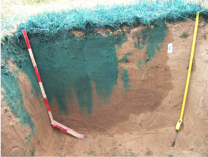
Figure 1.2: Demonstration of wetting front instability. The experiment was realized at Mlaky II near Sekule in 2010 [76]. Water was supplied across the top boundary at a small constant rate. Substantial part of the matrix remained dry after long time of steady infiltration.
