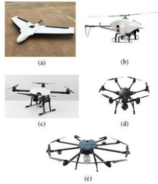
a) Fixed wings, b) single motor, c) quadcopter, d) hexacopter, e) octocopter (Source 3)
