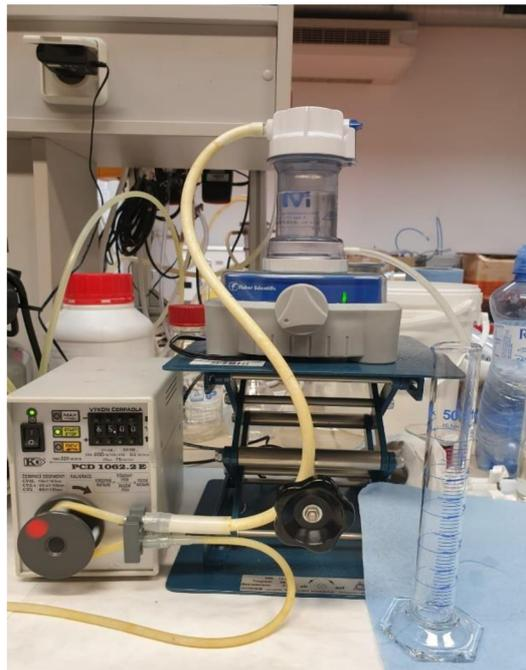
Figure 15. Water flux testing machine.
