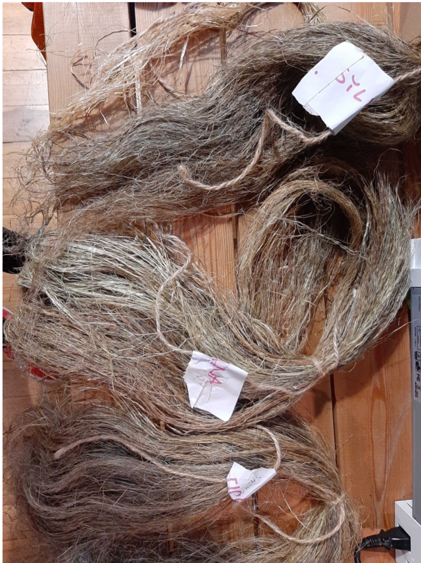
A demonstration photo of some of the varieties after the decortication. Sylvana harvested in January (top), Sylvana harvested in December (middle) and Santhica harvested in December (bottom), which was chosen for further assessments.
