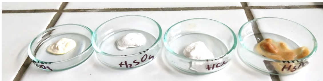
Fig. 4.5: Acid digestion with different acids. Preparation followed general procedure 3.3.2.1, biomass concentration was 38 % CDW, concentration of acid in reaction mixture was 0.4 mol/l and the mixture reacted 3 h/95 °C.
