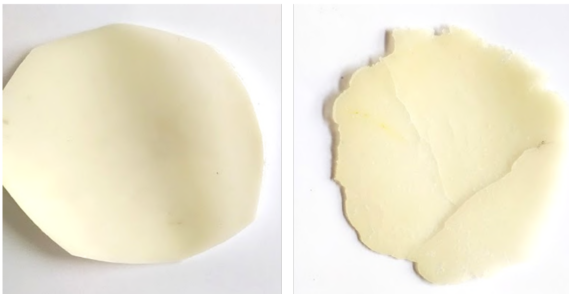
Fig. 4.18: PHB samples after melting at 190 °C/5 min and cooling. Left: commercial PHB, right: PHB obtained by soap-based digestion. The sample spontaneously cracked upon cooling.
