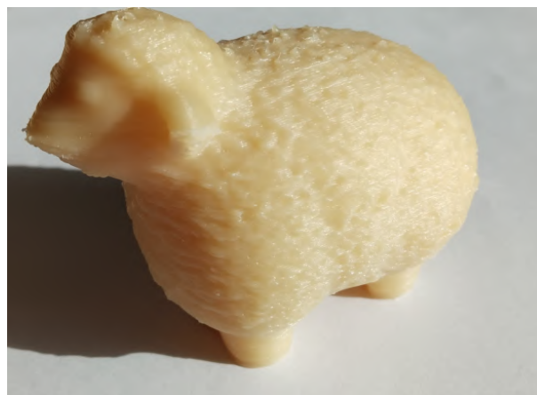
Fig. 4.22: 3D printed object made from our PHB. The polymer came from soap-based digestion and was stabilized with 2 % succinic anhydride before melt processing
