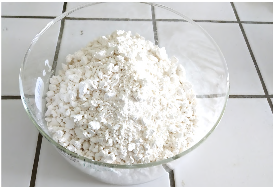
Fig. 4.14: PHB isolated by soap-based digestion
