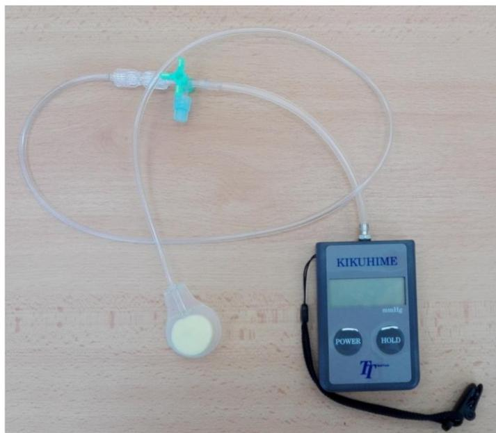
*Figure 14: The Kikuhime pressure measuring device*
