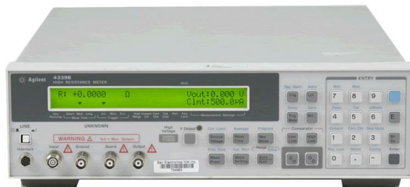
obr. 15: Megaohmmetr Agilent 4339B [36]
