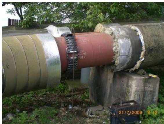
Obr. 4.9 Metoda Guided Waves [48]
