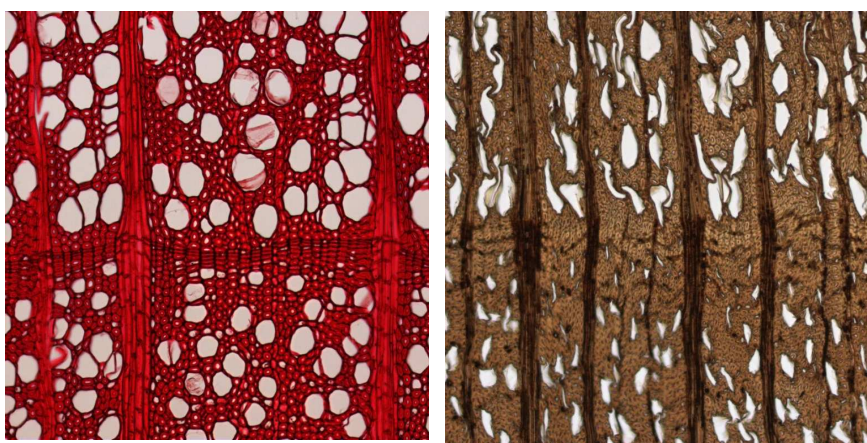
Paper I. Fig 4 Microstructure pictures of untreated beech wood (on the left side) and Lignamon (on the right side); magnification of approximately 100x
