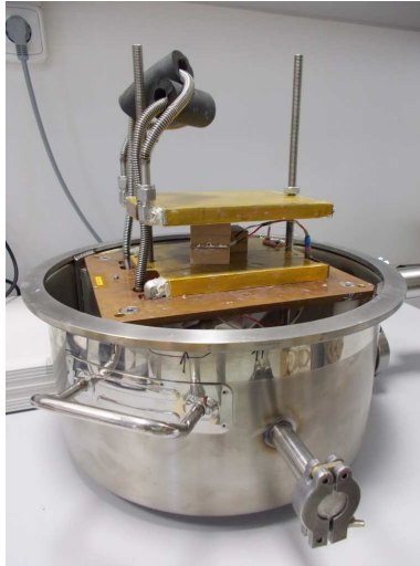
Paper III. Figure 2 Opened chamber of RT-Lab device based on pulse-transient method
