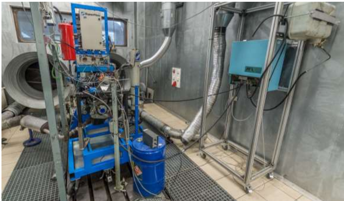
Figure D.2 Instrumented engine in the test cell
