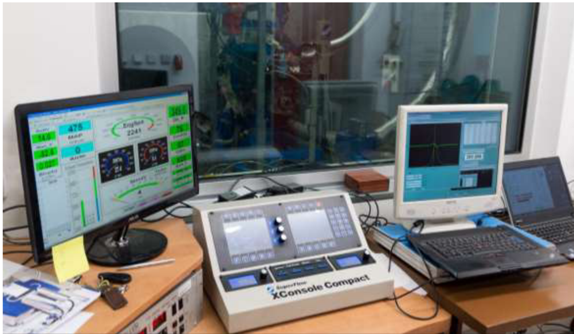
Figure D.1 Engine test cell control room
