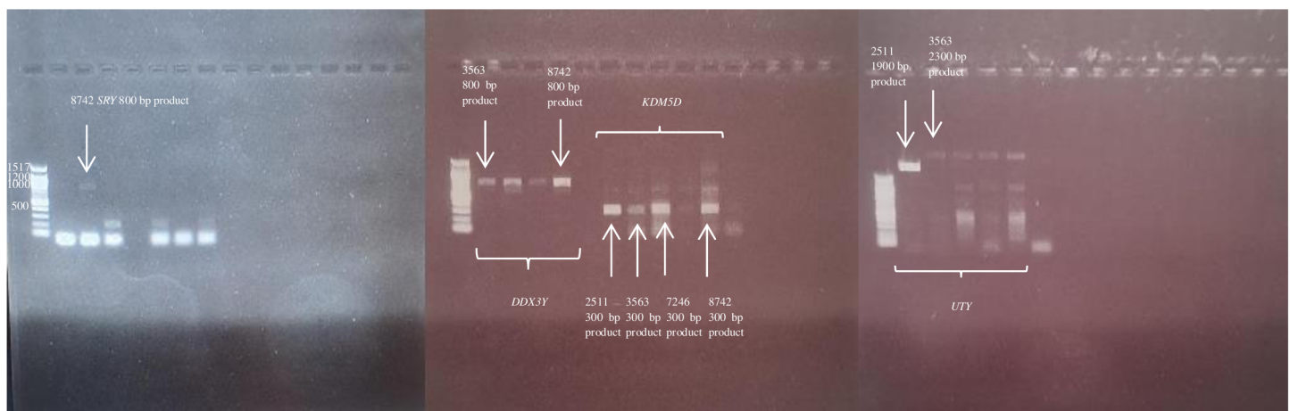
Figure 8: Examples of products which were purified and sent for Sanger sequencing obtained through PCR with 33, 34, 32, 32 cycles and 60 °C, 61 °C, 64 °C, 66 °C as annealing temperatures for SRY , DDX3Y , KDM5D and UTY respectively
