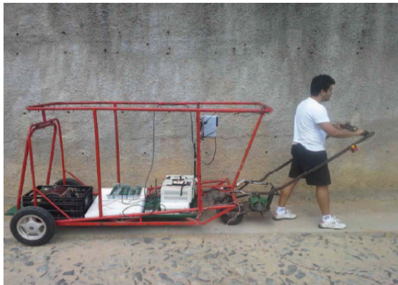
Figure 3.2: Mechanical traction system for electrical load cart developed by Silva et al. [43]
