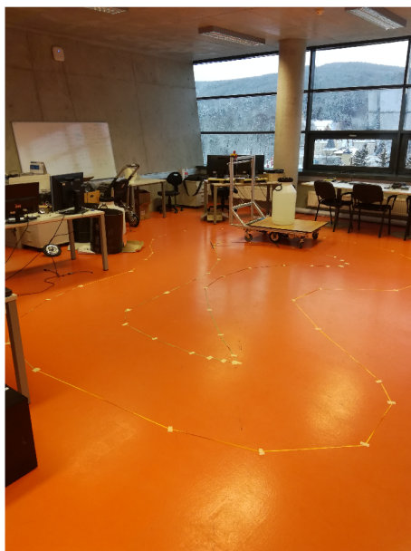
Figure 10.15: Predefined track. Setup for m_{load+cart} = 103[kg]
