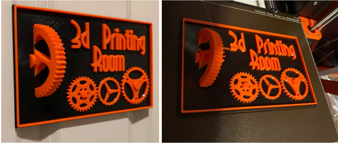
Figure 7: Sample object printed using the pause and swap printing method. Source: MikeL via Printables (2022)
