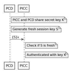
Figure 10: Simplified authentication used in model
