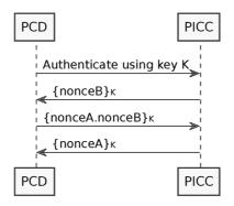
Figure 9: Three-pass authentication example
