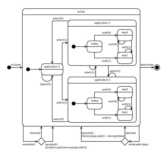
Figure 4: UML state machine describing basic Mifare DESFire behavior
