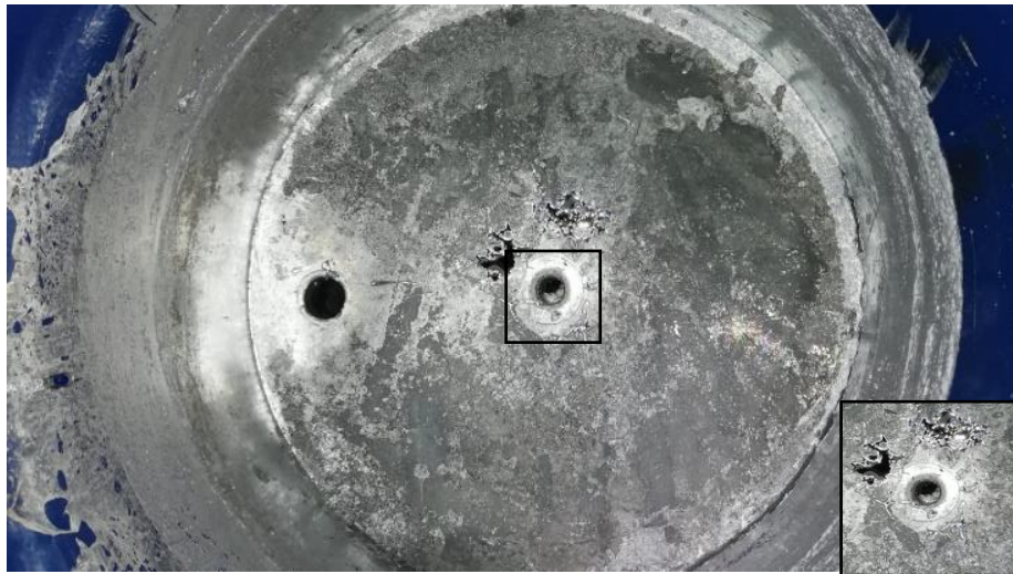
Figure 5.1. Clogging in the SEN near 'tundish' outlet
