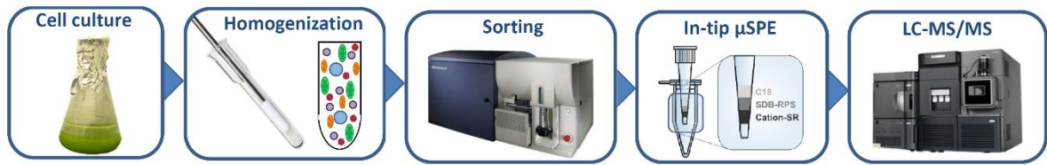
Figure 11 Workflow of organelle sorting. From left to right: (i) 14-days-old Arabidopsis cell suspension culture, (ii) cell homogenization and staining with fluorescent dyes (20 min), (iii) FACS instrument for analysing and sorting the organelles (30 min), (iv) phytohormone in-tip micro solid-phase extraction ( \mu SPE) purification (3 h), and (v) liquid chromatography-tandem mass spectrometry (LC-MS/MS) analysis (10 – 15 min).
