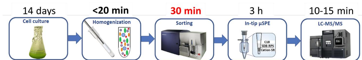
Figure 2. Summarized workflow of FAMOS with specified duration of each step as follows: (i) growth of plant cells in suspension culture, (ii) sample homogenization with a Potter-Elvehjem tissue grinder and staining with fluorescent dyes, (iii) fluorescence-activated multi-organelle sorting (FAMOS), (iv) phytohormone isolation by in-tip micro-solid phase extraction (in-tip \mu\text{SPE} ), and (v) liquid chromatography-tandem mass spectrometry (LC-MS/MS) analysis. A detailed workflow is shown in Figure S2.
