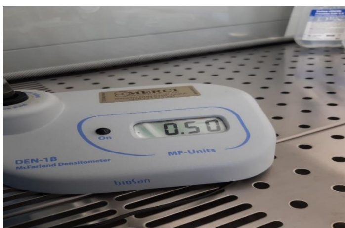
Figure 8. McFarland standard.DEN-1B Densitometer (suspension turbidity detector)
