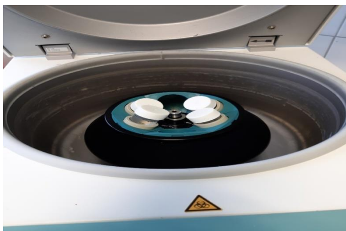
Figure 7. Centrifugation of chitosan and Cannabis extract nanoparticles (source: author)
