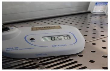
Figure 8. McFarland standard.DEN-1B Densitometer (suspension turbidity detector)
