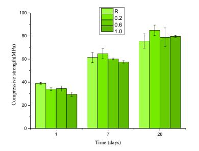
Fig. 21.: Compressive strength of GBFS activated by WG with a modulus of 0.5 with the addition of lignosulfonate
