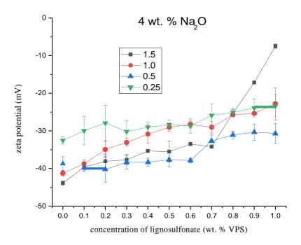
Fig. 28: Dependence of the zeta potential ( $\zeta$ ) on the wt.% of the addition of lignosulfonate in the GBFS mixture activated by WG with different modules
