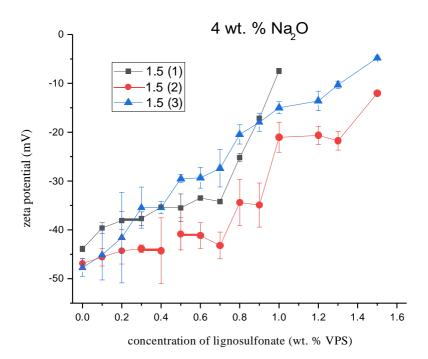
Fig. 29: Dependence of the zeta potential ( $\zeta$ ) on the wt.% of the addition of lignosulfonate of the GBFS mixture activated by WG with a modulus of 1.5
