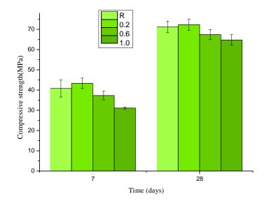
*Fig. 23.*: Compressive strength of GBFS activated with Na<sub>2</sub>CO<sub>3</sub> with the addition of lignosulfonate
