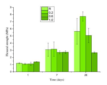
*Fig. 18.*: *Flexural strength of GBFS activated by WG with a modulus of 1.5 with the addition of lignosulfonate*
