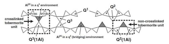
Fig. 4.: Myers model of alkali-activated blast furnace slag [3]
