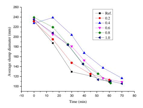
Fig. 12.: Influence of lignosulfonate plasticizer on workability of water glass activated GBFS with silicate modulus of 1.0
