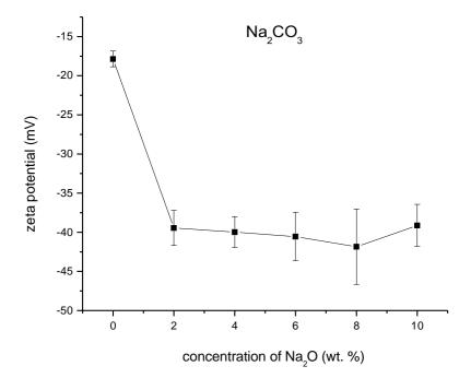
*Fig. 30*: Dependence of the zeta potential ( $\zeta$ ) on the wt.% of Na<sub>2</sub>O activated by Na<sub>2</sub>CO<sub>3</sub>
