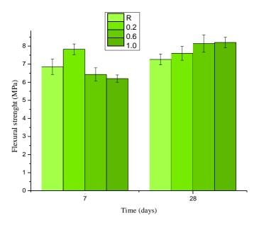
Fig. 24: Flexural strength of GBFS activated with Na<sub>2</sub>CO<sub>3</sub> with the addition of lignosulfonate
