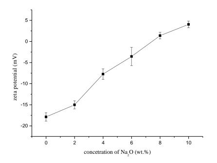
*Fig.* 25: Dependence of the zeta potential ( $\zeta$ ) on the wt.% of Na<sub>2</sub>O in NaOH activator
