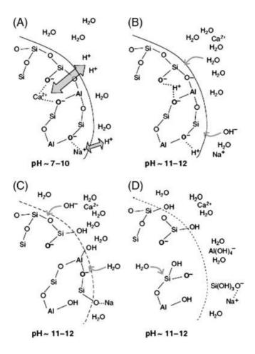
**Fig. 5**. : Mechanism of dissolution of aluminosilicate glass during the early stage of the reaction: (A) exchange of H<sup>+</sup> ions for Ca<sup>2+</sup> and Na<sup>+</sup>, (B) hydrolysis of Al–O–Si bonds, (C) depolymerization of the glass network and (D) release of Si and Al [17]
