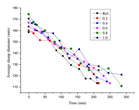
Fig. 14.: Influence of lignosulfonate plasticizer on workability of GBFS activated by Na<sub>2</sub>CO<sub>3</sub>
