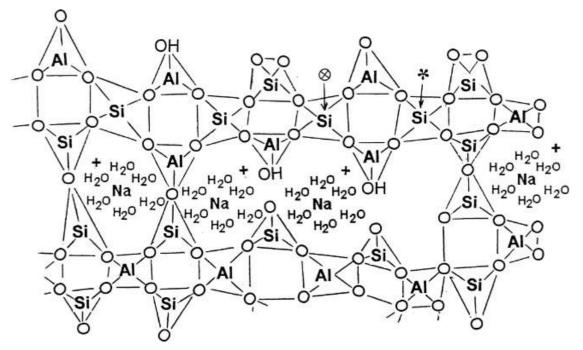
Fig. 3: Barbarosian model of geopolymer alkali-activated material [4]
