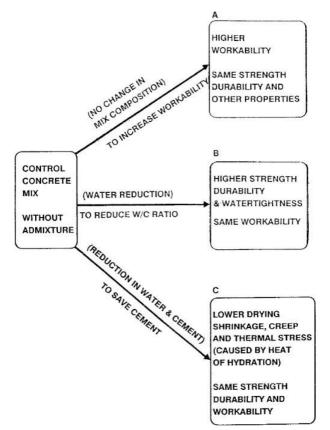
Fig. 6.: Influence of superplasticizer on concrete mixtures [18,20]
