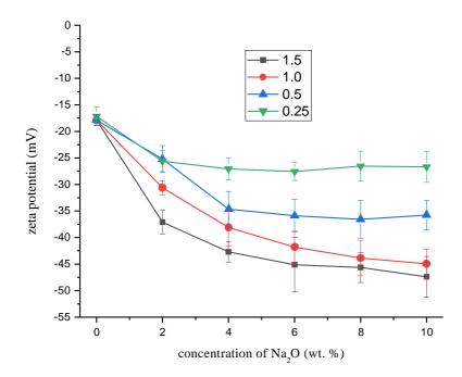
Fig. 27: Dependence of the zeta potential ( $\zeta$ ) on the wt.% of Na<sub>2</sub>O of WG activator with different modules
