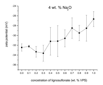
*Fig. 31.*: Dependence of the size of the zeta potential (ζ) on the addition of wt.% of lignosulfonate in the GBFS mixture activated by Na<sub>2</sub>CO<sub>3</sub>
