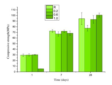
Fig. 17.: Compressive strength of GBFS activated by WG with a modulus of 1.5 with the addition of lignosulfonate
