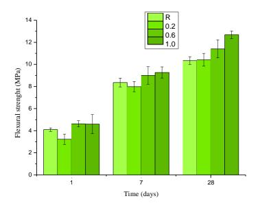
Fig. 16.: Flexural strength of GBFS activated with NaOH with the addition of lignosulfonate
