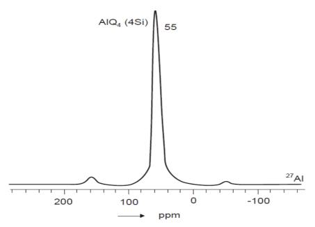
Fig. 1: NMR MAS <sup>27</sup>Al of "real" geopolymer [6,7]
