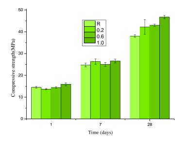
Fig. 15.: Compressive strength of GBFS activated with NaOH with the addition of lignosulfonate
