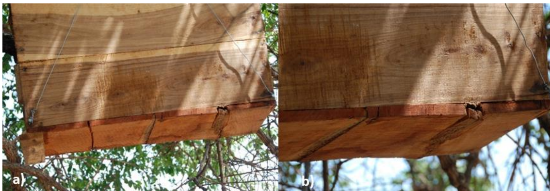
Figure 8 Wood dried on the hive and created gaps
