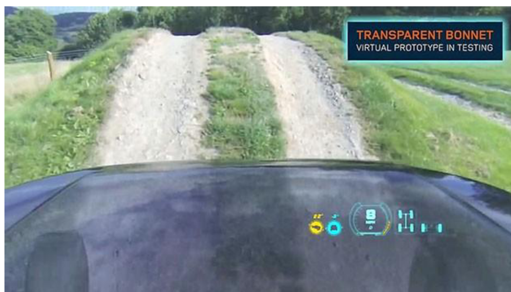
Obr. 14 Technologie Transparent hood automobilky Land Rover [12]
