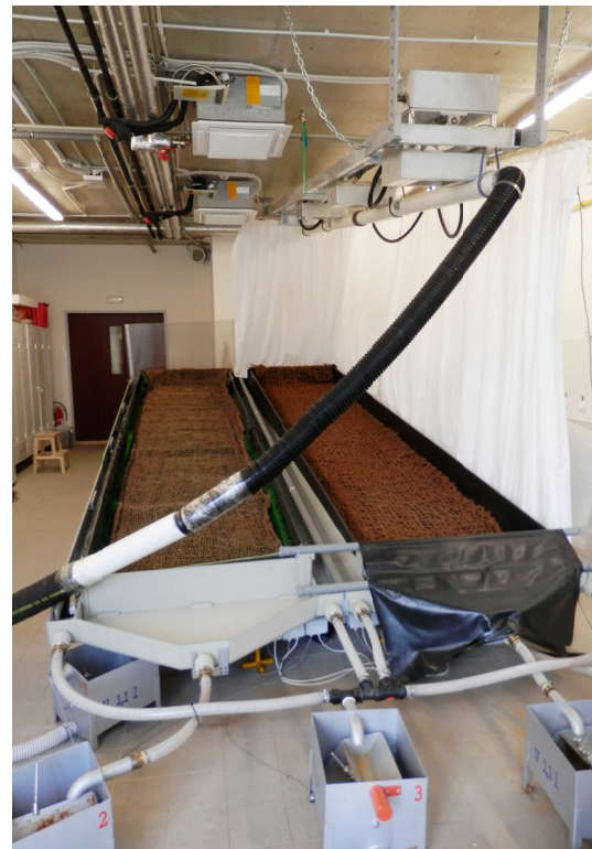
Figure 1. A Norton Ladder Rainfall Simulator is positioned above test beds with mechanical toggle flow meters. A C400 erosion control net is spread over the test bed.
