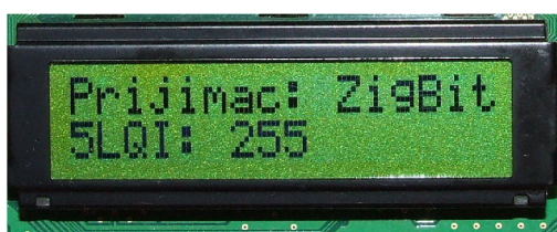
Obr. 8.19: LQI ( Link Quality Indicator ) pro a) ZigBee b) XBee
