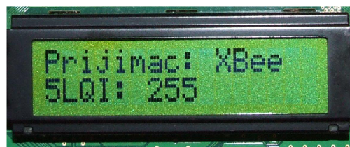
Obr. 8.19: LQI ( Link Quality Indicator ) pro a) ZigBee b) XBee
