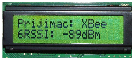
Obr. 8.20: RSSI ( Received Signal Strength Indicator ) pro a) ZigBee b) XBee
